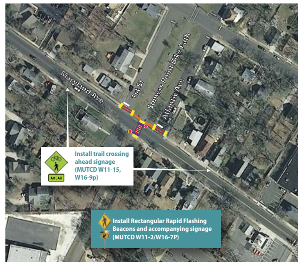
Figure 8-50 | Secondary Arterial Trail Crossing Template
